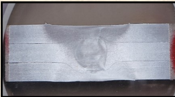
Friction Stir Welding for Additive Manufacturing Macro (3mm thick plate) and fracture location.
